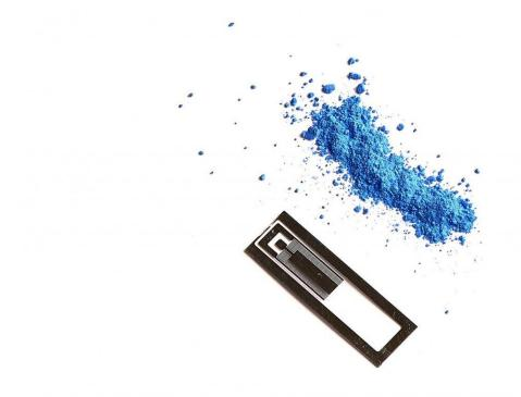
An acoustically-created MOF, with the microchip that produced the high-frequency sound waves used in the process. Credit: RMIT University
