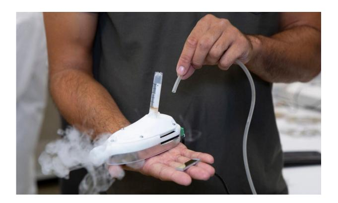
The patented 'Respite' nebuliser uses high-frequency sound waves to precisely deliver drugs to the lungs. Credit: RMIT University
