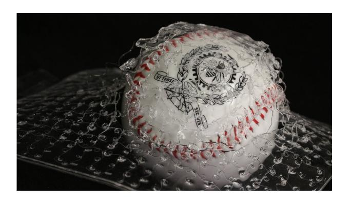
Polycarbonate webs synthesized using additive manufacturing absorb up to 96% of impact energy. Credit: Shibo Zou
