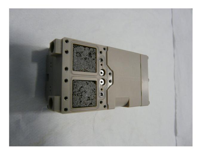
A biomining reactor containing small slices of basalt rock. Credit: Charles Cockell
