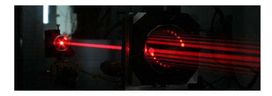
Researchers have developed an extremely sensitive, yet simple optical method for detecting formaldehyde. Their approach is based on multipass spectroscopy, which introduces a laser through a small hole in a mirror. The laser light then bounces back and forth between mirrors, creating interaction lengths with the sample that are tens or hundreds of times the length of the cell. Credit: Mateusz Winkowski, University of Warsaw
