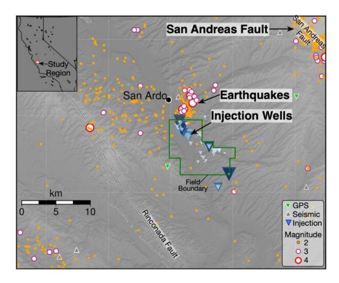
The stresses from injecting water can trigger earthquakes several miles from the well itself. The blue triangles scale with each well's injection rate. Credit: Thomas Goebel/University of Memphis, CC BY-ND
