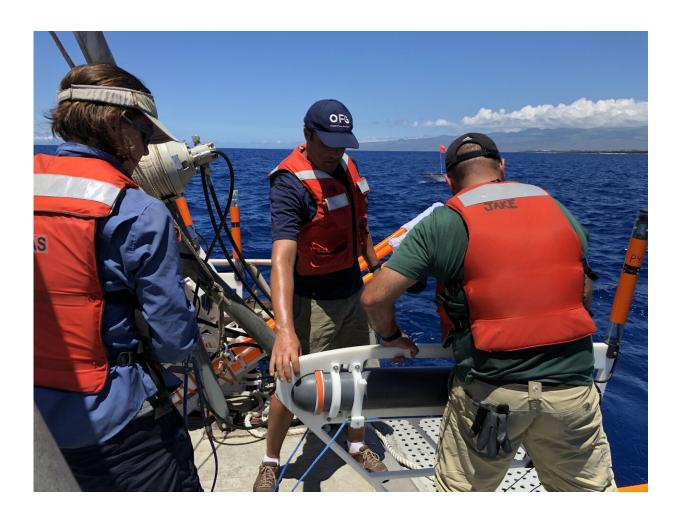
Eric Attias (middle) deploying the surface-towed marine controlled-source electromagnetic (CSEM) system off of Hawai'i Island. Credit: University of Hawai'i
