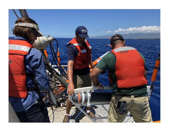
Eric Attias (middle) deploying the surface-towed marine controlled-source electromagnetic (CSEM) system off of Hawai'i Island. Credit: University of Hawai'i
