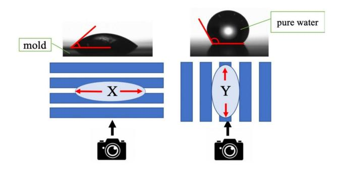
Measuring how a drop of water makes contact with the grooves of a nanolithography mold to find out how worn out the mold is. Credit: Jun Taniguchi, Tokyo University of Science
