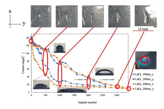
Plot of the contact angle along the parallel (y) and perpendicular (x) directions versus number of uses of the mold. The mold becomes defective when the contact angle along the vertical direction becomes equal to the stable minimum value along the perpendicular direction. Credit: Jun Taniguchi, Tokyo University of Science
