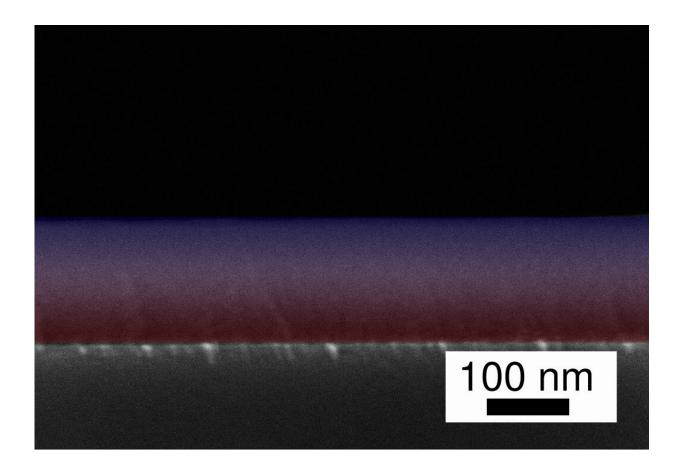
Using an elaborate process, the research team has joined two polymers at the nanoscale in a flowing process: The transition from PV3D3 to Teflon (PTFE) in the scanning electron microscope image of the gradient layer is marked here as the transition from red to blue. Credit: Kiel University
