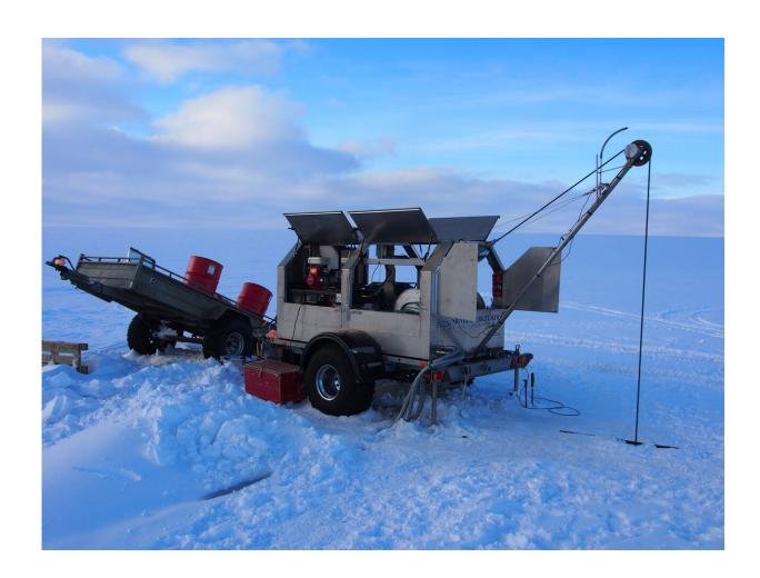
The hot water drill used to drill through the glacier to the subglacial lakes. The drill stem is hundreds of meters below in the ice, suspended on a rubber hose through which hot water is pumped down. Credit: Eric Gaidos
