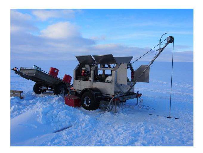
The hot water drill used to drill through the glacier to the subglacial lakes. The drill stem is hundreds of meters below in the ice, suspended on a rubber hose through which hot water is pumped down. Credit: Eric Gaidos
