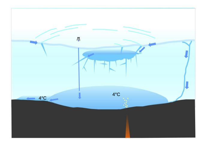
Illustration of the water movement that may have triggered the flood of June 2015 (arrows indicate flow direction): the subglacial lake, warmed to 4 C by geothermal input, the perched reservoir fed by summer melt through the firn layer, a water-filled system of crevasses and conduits (moulins), our borehole, and the outlet under the ice dam. Credit: Gaidos, et al. (2020)
