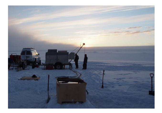
In June 2015, a team led by Gaidos used hot water to melt a hole through 250 meters of ice to sample a lake beneath a glacier in Iceland. Credit: Eric Gaidos
