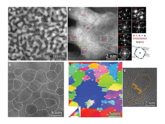
Microstructures of the as-prepared Cu sample with extremely fine grains. (A) A typical bright-field TEM image. (B) (Left) A magnified image of a selected area in (A). Dashed lines represent {111} planes and solid lines show CTBs. (Right) Corresponding FFT images of grains (G1, G2, G3, G4, and G5) labeled in the
