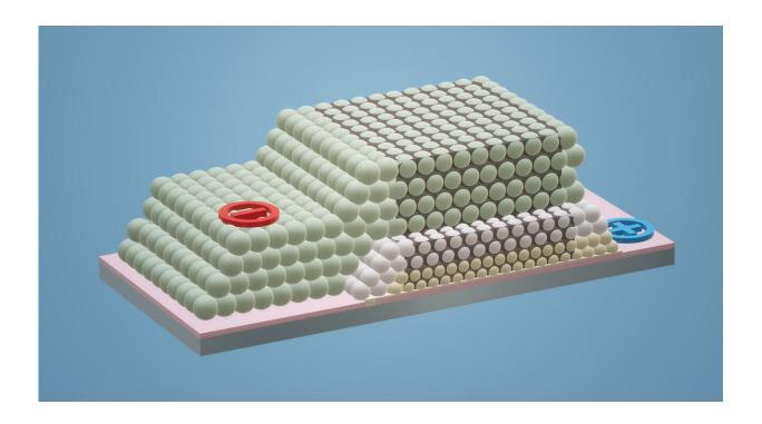
The triple oxide mesoporous indium tin oxide perovskite-based solar cell structure. Credit: Avi Schneider.
