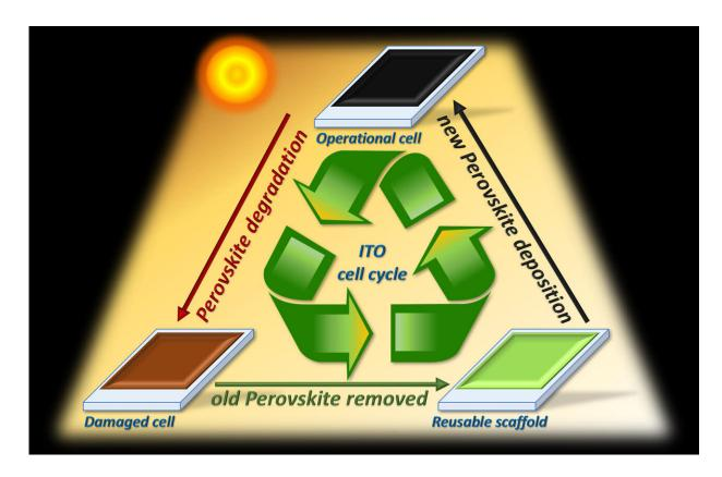
A scheme of the recycle process, which is unique for the mesoporous indium tin oxide perovskite-based solar cell. Credit: Avi Schneider.
