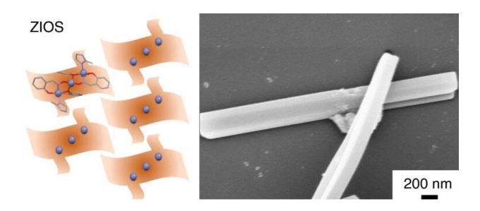
From left: Schematic diagram of a ZIOS network; and a SEM (scanning electron microscopy) image of a ZIOS-copper sample on a silicon wafer. Credit: Berkeley Lab
