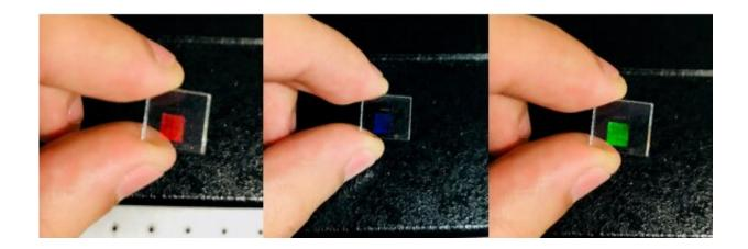
A demonstration of optical effects made possible using the nanoscale assembly method to align gold nanorods within a material. Different colours become visible to the observer as the angle of the prototype device changes. Credit: Heyou Zhang (Exciton Science)
