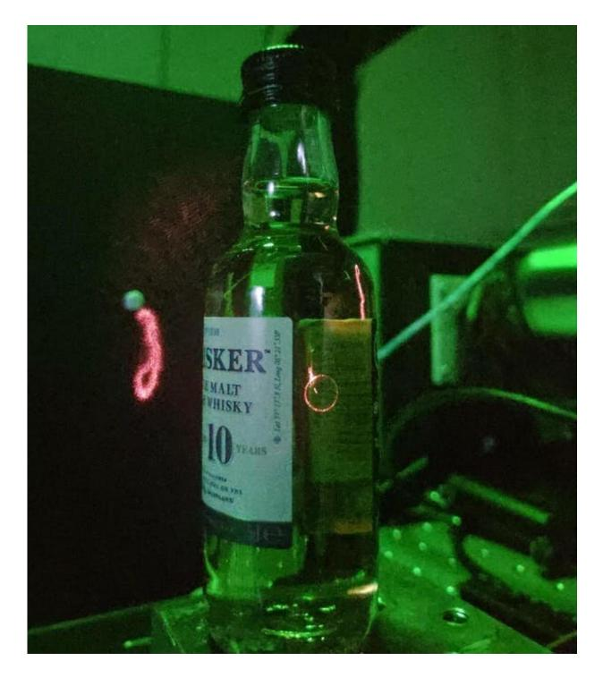
A special cone-shaped laser ensures the signal from the glass bottle does not interfere with the measurement of the liquid inside. Credit: University of St Andrews, Author provided
