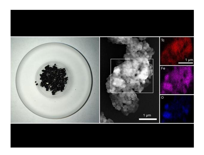
Iron granules (left) after one month of contact with technetium. Viewed under a scanning electron microscope, the red spots (top right) indicate that technetium is now retained by the iron's newly formed mineral phase. Credit: Daria Boglaienko | Pacific Northwest National Laboratory
