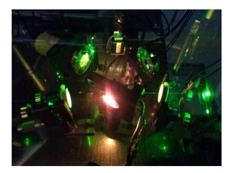
Potential applications of research conducted at the University of São Paulo include high-precision metrology and information encoding (pump laser for production of quantum-correlated light beams). Credit: Marcelo Martinelli / IF-USP
