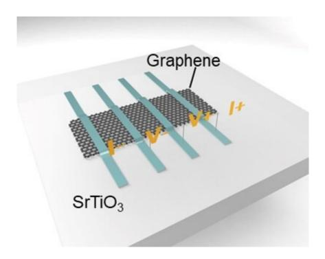
This illustration shows how strontium titanium oxide is combined with graphene strips. The combination opens up a new path to memristive heterostructures combining ferroelectric materials and 2D materials. Credit: Banerjee lab, University of Groningen
