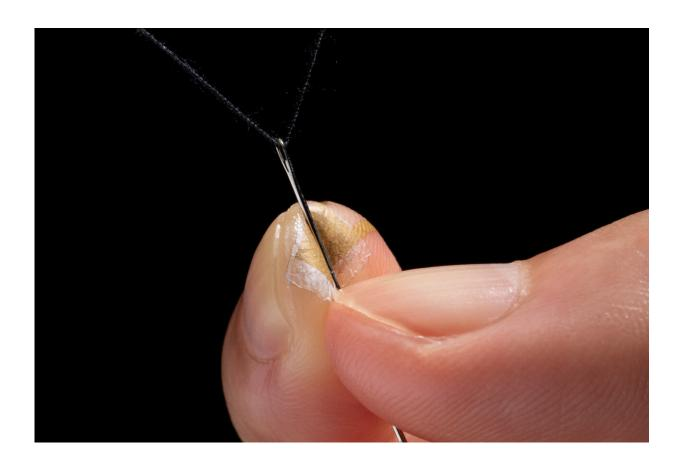
The polyurethane and gold sensor can resist shear forces and rubbing. Credit: © 2020 Someya et al.
