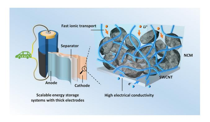
Thick electrodes with single-walled carbon nanotubes (SWCNTs) for scalable energy storage systems. Credit: Zhengyu Ju and Guihua Yu
