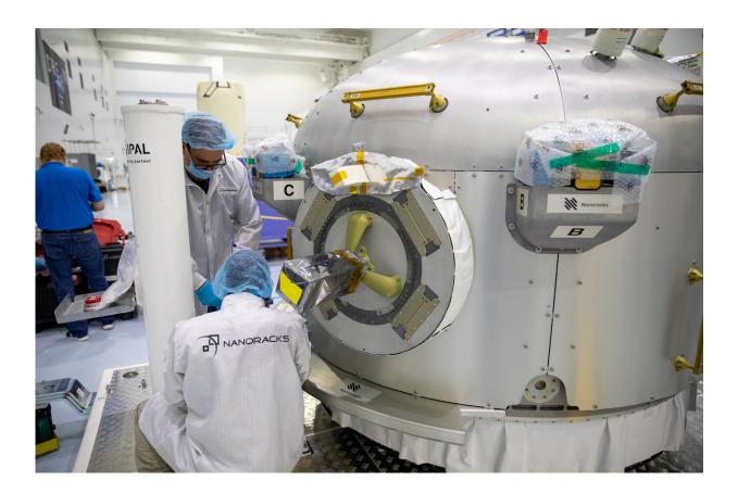
Technicians work on the Nanoracks Bishop Airlock inside the Space Station Processing Facility at NASA's Kennedy Space Center in Florida on Sept. 29, 2020, preparing the facility for its flight to the International Space Station. The first commercially funded airlock for the space station provides payload hosting, robotics testing, satellite deployment, and more. Credit: NASA/KSC
