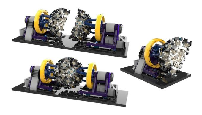
This set of renderings shows the completed GRETA array (top and bottom left) and half of the completed array (right). The detector is designed to open up, with each half sliding on tracks. Samples can be placed at the center of the spherical array. The completed array will contain 120 high-purity germanium crystals. Credit: GRETA collaboration
