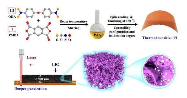
Fig.1. Schematic illustration for the improved laser inducing growth process of ultra-thick 3D graphene frameworks with hierarchical pores. Credit: LI Nian
