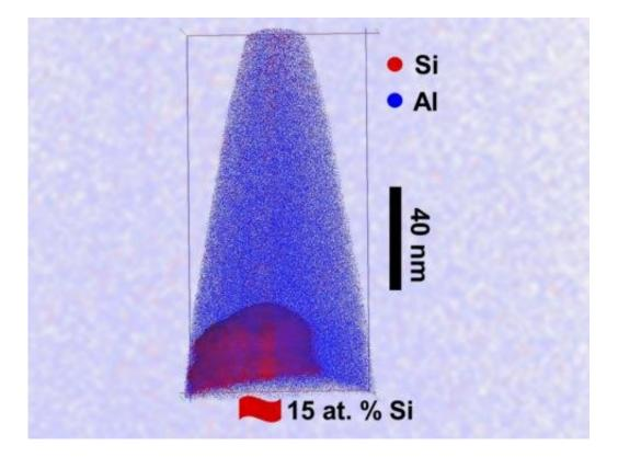
Atom probe tomography reveals the unique distribution of silicon (red) inside a highly refined aluminum matrix (blue). This distribution at the nanoscale is achieved by shear deformation, which leads to the alloy's higher strength. Credit: Arun Devaraj | Pacific Northwest National Laboratory
