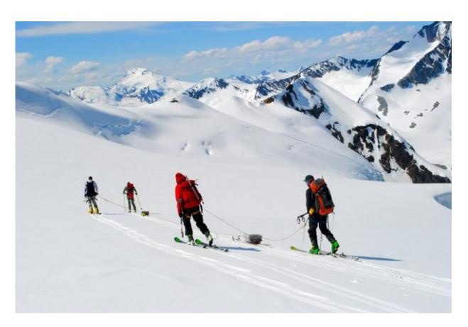
Ben Pelto's team of glaciologists during their fieldwork expedition to collect glacier thickness data. They are seen towing the pair of ice-penetrating radar devices on skis. Credit: Jill Pelto
