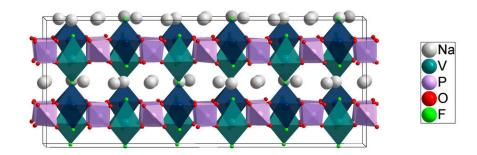
The low-temperature structure of NVPF [Na3V2(PO4)2F3] solved in this work. Calculations from Lawrence Berkeley National Laboratory suggest that the sodium atoms (white) can move most easily in the planes between the cation sites of vanadium (teal) and phosphorus (mauve) atoms during battery use. Credit: Brookhaven National Laboratory
