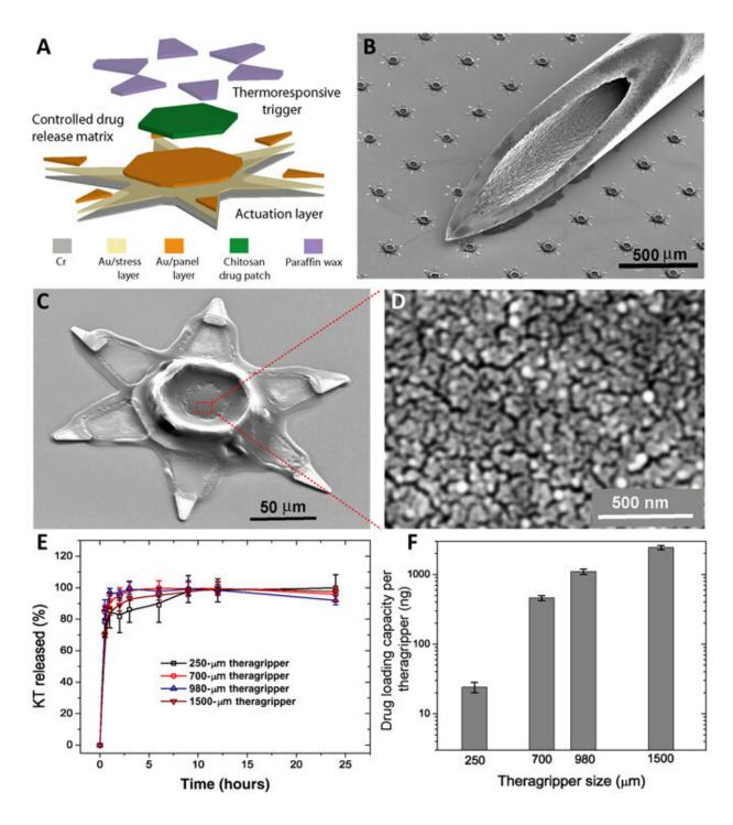
Parallel fabrication of the theragrippers and their in vitro drug loading and release characteristics. (A) Functional block diagram illustrating the microfabrication steps for an array of theragrippers, showing the actuation layer, drug-eluting layer, and the thermoresponsive trigger. (B) SEM image showing theragrippers next to the tip of a 22-gauge hypodermic needle. The theragrippers
