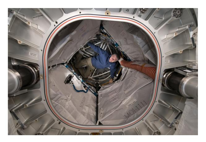
ESA astronaut Paolo Nespoli completes some tests in the Bigelow Expandable Activity Module, or BEAM, on the International Space Station. Credit: ESA/NASA
