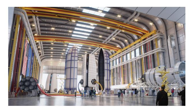
Architectural firm Skidmore, Owings & Merrill has designed a semi-inflatable Moon Village habitat. The habitat would be completely equipped and tested on Earth, before it is erected and inflated on the lunar surface. With a mass exceeding 58 tonnes, the habitat would utilise a heavy-lift launcher such as a future upgrade of SLS or the SpaceX Starship. Credit: SOM
