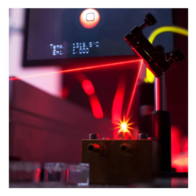
The laser-heated aerodynamic levitation furnace which Sossi's group used in the experiments. Credit: IPGP
