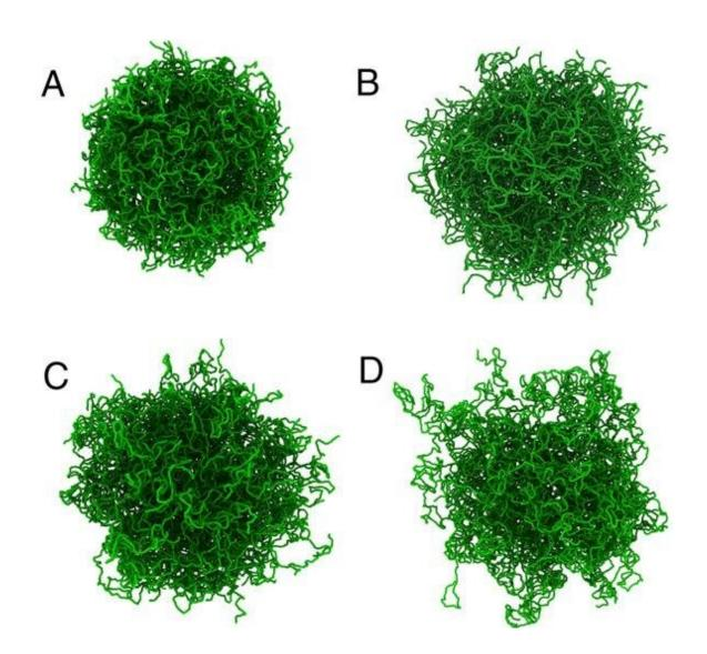
Simulation snapshots of swollen microgel particles. (Top) Microgels that have a uniform cross-link distribution, and (Bottom) microgels that have a Gaussian cross-link distribution. Credit: Georgia Tech
