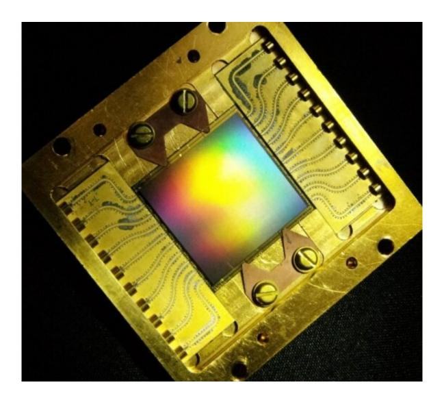
The 20440 pixel MKID device designed for MKID Exoplanet Camera is the highest pixel-count superconducting detector array at any wavelength. Credit: Image courtesy of researchers
