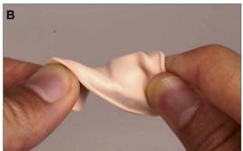
Wireless, soft, skin-interfaced sensor platform designed for mounting on the suprasternal notch. The wearable device is leading to better understanding of droplet dynamics in the COVID-19 pandemic. Credit: KunHyuk Lee, Northwestern University
