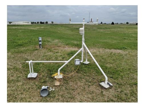
3-D-printed weather station initial installation in the field. Credit: Argonne National Laboratory
