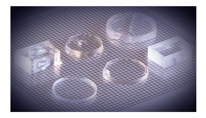
An array of polished, 3D printed gradient refractive index lenses made of titania-
