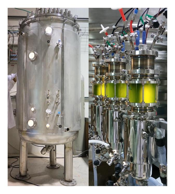
A large bioreactor (left) and smaller labscale bioreactors (right). Credit: Yonatan Golan, Brevel
