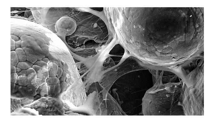
This image shows cells adhering to a titanium alloy created by cold-spray 3D printing, which demonstrates the material's biocompatibility. Credit: Cornell University
