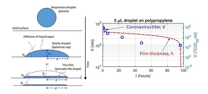
Schematic of a thin liquid film drying on a surface and comparison of timevarying film thickness with a coronavirus titer (the lowest concentration of virus that still infects cells) on plastic. Credit: R. Bhardwaj and A. Agrawal
