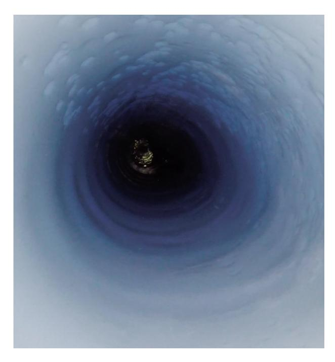
View down an ultra-clean hot water borehole drilled into Mercer Subglacial Lake, a freshwater lake located more than 1000 metres beneath the Antarctic Ice Sheet. The lake is hydrologically active, meaning water flows through it to the coast, much like lakes on land. Meltwater from this lake is highly enriched in biologically essential trace elements like Iron. Credit: Katryn Kasic, Montana State University
