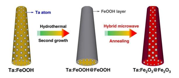
Figure 1. Schematic synthesis procedure of Ta:Fe2O3@Fe2O3 homojunction nanorods. Using hybrid microwave annealing, hematite homojunction nanorod is synthesized by hydrothermal regrowth of thin FeOOH layer on Ta:FeOOH nanorods. Credit: Jae Sung Lee, UNIST
