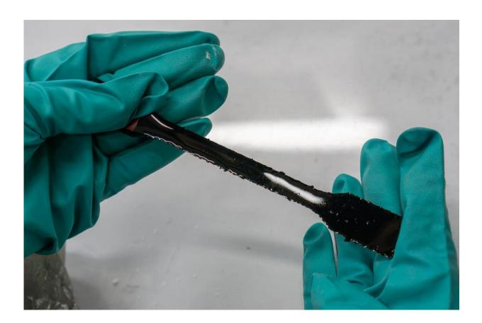
Carbon-nanocomposite after finishing the molding process. The sample will be tested for piezoresistive response after minor finishing touches. These materials can be shaped into almost any size and form. Credit: The image was taken in the Laboratory of Micro and Nano Mechanics, CDMM at Skoltech.
