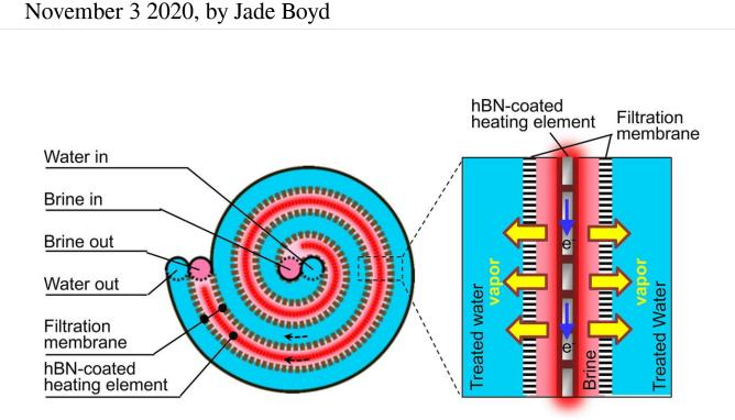
Rice University's desalination technology for hypersaline brine features a central passage for heated brine that is sandwiched between two membranes. A stainless steel heating element produces fresh, salt-free water by driving water vapor through each membrane. A coating of the 2D nanomaterial hexagonal boron nitride (hBN) protects the heating element from the highly corrosive brine. Credit: Kuichang Zuo/Rice University
