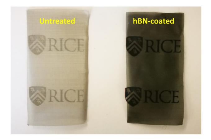
Rice University engineers created a robust heating element for desalinating highly corrosive industrial-strength brine by adding a protective coating of the 2D nanomaterial hexagonal boron nitride to a commercially available stainless steel mesh. Credit: Kuichang Zuo/Rice University
