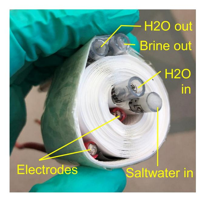
A coiled distillation membrane system for desalinating hypersaline brine. Rolling the system into a coil demonstrated the possibility of adopting a common space-
