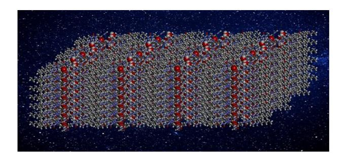
Artificial water channels inserted into a polyamide membrane © Mihail Barboiu, Institut Européen des Membranes. Credit: CNRS/ENSC Montpellier/University of Montpellier
