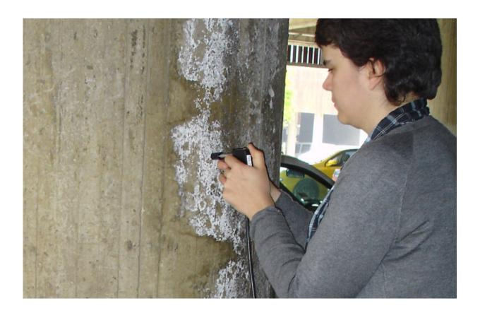
Dr Iratxe Ibarrondo using portable high-resolution spectroscopic techniques to analyze the impact on 20th-century construction materials of the environment and biological conditions in the surrounding area. Credit: Iratxe Ibarrondo/UPV/EHU.
