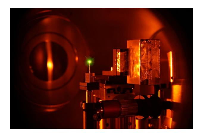
A material sample is placed in the target chamber of GSI's high-performance laser PHELIX. With the aid of the high-intensity laser beam protons are then accelerated out of its back-surface. Credit: V. Bagnoud, edit: P. Boller / GSI
