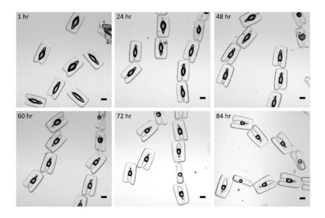
Images showing the volume can be maintained over several days inside U-shaped cups that are each about a half-millimeter in length. A slow reduction in the volume of drops is presumably due to dissolution of water in the oil phase and evaporation over time. Credit: Di Carlo Research Group/UCLA
