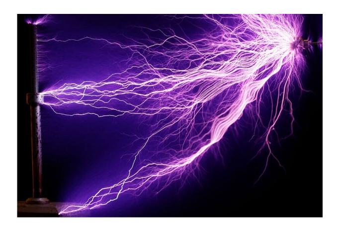
Arcs of electricity generated by a Tesla coil. Credit: Airarcs/CC BY-SA 3.0
