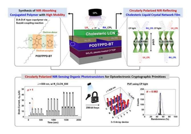
A Schematic Diagram of the Major Strategies for the Development of Near-infrared Radiometric Sensitivity Photovoltaic Transistor. Credit: Korea Institue of Science and Technology (KIST)
