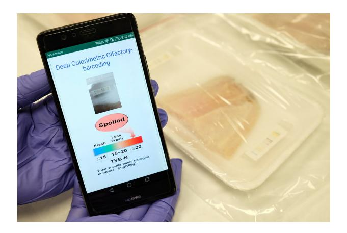
The e-nose comprises a 'barcode' that changes colour due to reactions with gases emitted by the decaying meat, and a barcode 'reader' in the form of a smartphone app powered by AI, and has been trained to recognise and predict meat freshness from a large library of barcode colours. Credit: Nanyang Technological University
