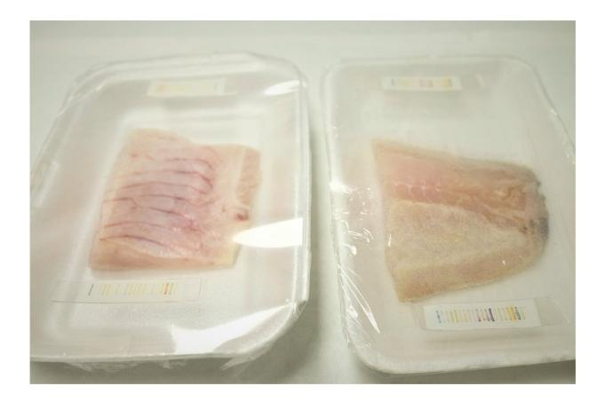
The barcode is attached to the underside of the PVC film that the meat is packaged in. Credit: Nanyang Technological University
