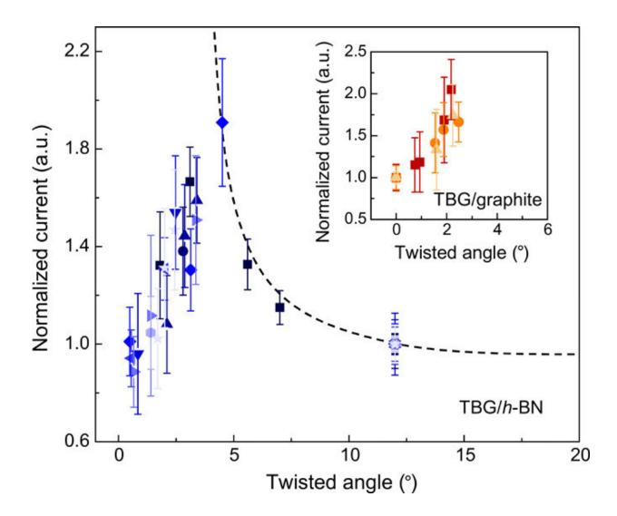
Dependence of vertical conductivity on twist angle. The relationship between the normalized current and the twist angle obtained on TBG/h-BN is shown. Data with the same symbol color and shape were obtained simultaneously from the same current image. The inset shows the relationship between current and twist angle obtained on twisted graphene on graphite, where the current values were
