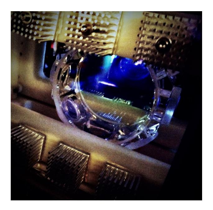
A 3 cm-long ensemble of cesium atoms laser-cooled in a glass chamber is used as a quantum memory. Credit: LKB
