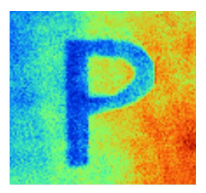
This infrared image shows that the P pattern pained with the Purdue radiative
